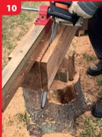
10 Cutting first plank.
