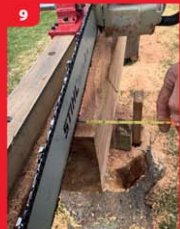
9 Measuring for board width.
