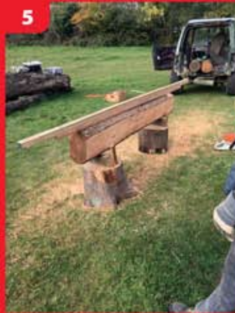
5 Simply turn GO2 MILL around on rail and cut the opposite side.
