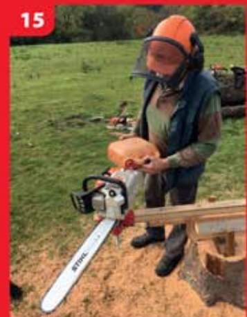
15 GO2 MILL positioned sideways to allow easy refueling.
