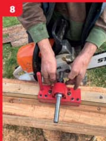
8 2.5mm per turn to determine plank width.
